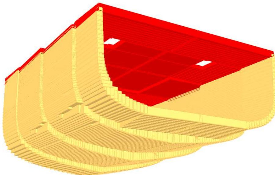
*Figure 2: FDS geometry model presenting the engine room of a small offshore patrol vessel, bulkheads are omitted from the visualization.*
