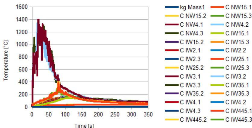
Figure 8: Temperature histories outside and inside structures with no sprinklers acting.
