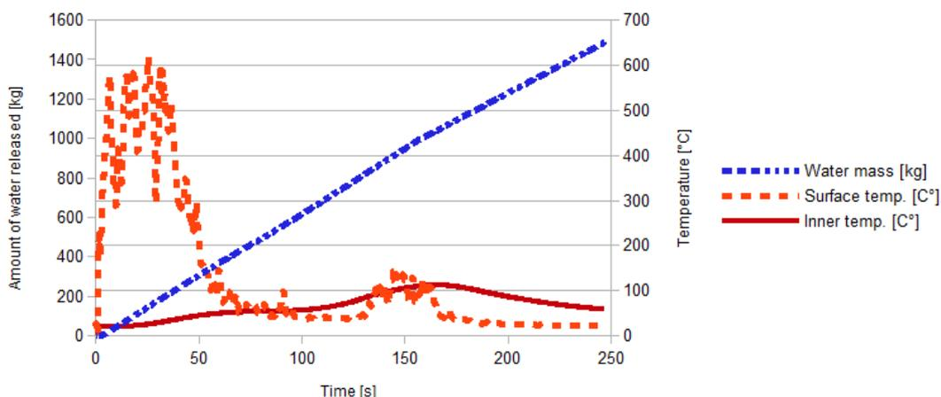
Figure 6: Histories of accumulated water and temperatures outside and inside structures.
