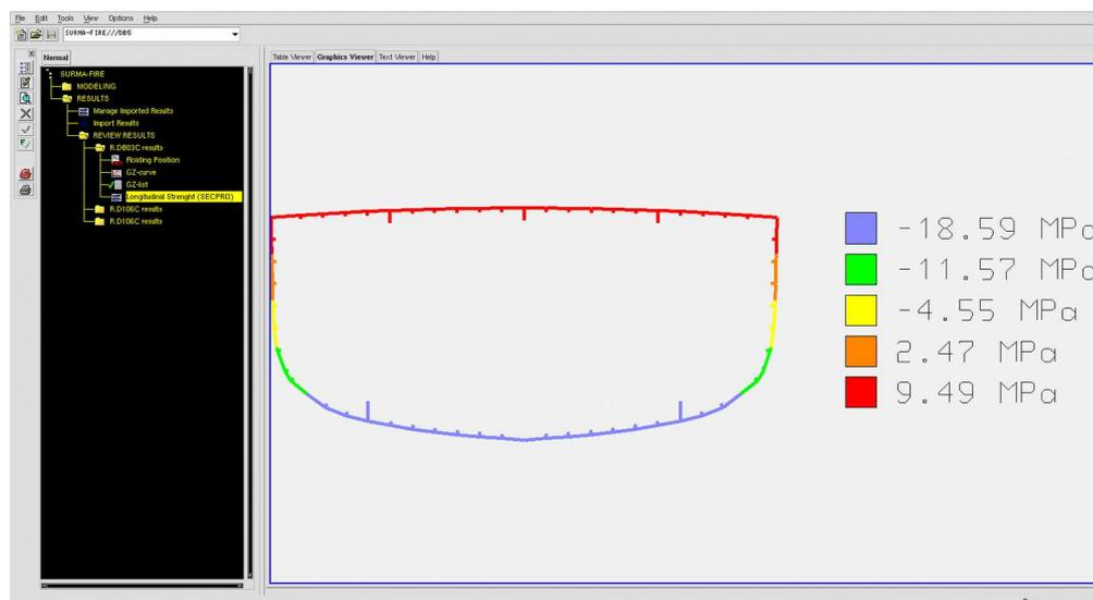
Figure 12: Longitudinal strength analysis are done using SECPRO, results viewed in manager
