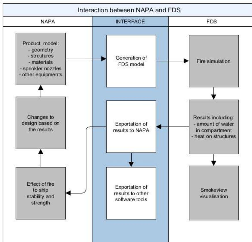
Figure 3: Integration of fire simulation and ship product model
